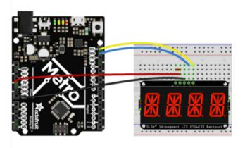
Board 5V to backpack Vio (long red wire) Board GND to backpack GND (black wire) Board SCL to backpack SCL (yellow wire) Board SDA to backpack SDA (blue wire) Backpack VIO to backpack VHi (short red wire)
