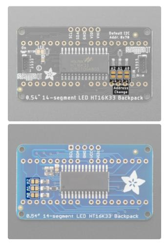
On the back of the board are **three address jumpers**, labeled **A0**, **A1**, and **A2**. These jumpers allow you to chain up to 8 of these boards on the same pair of I2C clock and data pins. To do so, you solder the jumpers "closed" in various combinations by connecting the two pads.
