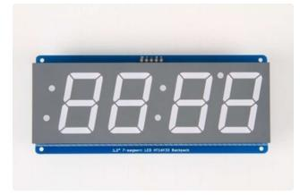
Remove the parts from packaging and place the LED matrix OVER the silkscreen side. DO NOT PUT THE DISPLAY ON UPSIDE DOWN OR IT WONT WORK!! Check the image below to make sure the 'decimal point' dots are in the same location as the ones on the silkscreen.
