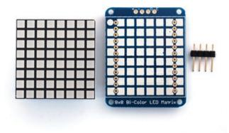
When you buy a pack from Adafruit, it comes with the fully tested and assembled backpack as well as a 8x8 matrix. You'll need to solder the matrix onto the backpack but its an easy task.
