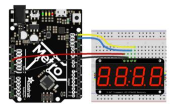
Backpack + (VCC) to microcontroller 5V (if using a board with 5V logic, otherwise use 3V for boards with 3V logic) (red wire) Backpack - (GND) to microcontroller GND (black wire) Backpack D (SDA) to microcontroller SDA (blue wire) Backpack C (SCL) to microcontroller SCL (yellow wire)
