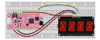
Board 5V to backpack Vio (red wire connected along the bottom of the Feather)
