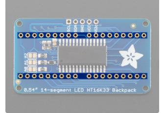
These two rows of through-hole pads are for soldering the alphanumeric LED displays onto the backpack. See the <u>Assembly page (https://adafru.it/11dU)</u> for details on attaching the displays properly.
