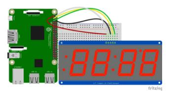
Raspberry Pi 3.3V to 7-Segment Display IO Raspberry Pi 5V to 7-Segment Display VIN Raspberry Pi GND to 7-Segment Display GND Raspberry Pi SCL to 7-Segment Display SCL Raspberry Pi SDA to 7-Segment Display SDA
