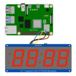
Raspberry Pi 3.3V to STEMMA QT red wire Raspberry Pi GND to STEMMA QT black wire Raspberry Pi SCL to STEMMA QT yellow wire Raspberry Pi SDA to STEMMA QT blue wire
