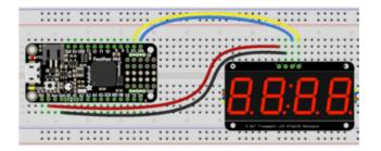
Microcontroller 3V to 7-Segment Display VIN (red wire) Microcontroller GND to 7-Segment Display GND (black wire) Microcontroller SCL to 7-Segment Display SCL (yellow wire) Microcontroller SDA to 7-Segment Display SDA (blue wire)
