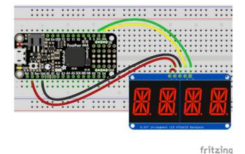
Microcontroller 3V to AlphaNumeric Display I2C VIN Microcontroller 3V to AlphaNumeric Display VIN Microcontroller GND to AlphaNumeric Display GND Microcontroller SCL to AlphaNumeric Display SCL Microcontroller SDA to AlphaNumeric Display SDA
