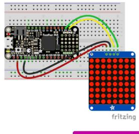
Microcontroller 3V to LED Matrix VIN Microcontroller GND to LED Matrix GND Microcontroller SCL to LED Matrix SCL Microcontroller SDA to LED Matrix SDA
