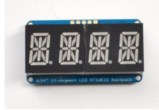
Remove the parts from packaging and place the LED matrices OVER the silkscreen side. DO NOT PUT THE DISPLAY ON UPSIDE DOWN OR IT WONT WORK!! Check the image below to make sure the 'decimal point' dots are on the bottom, matching the silkscreen.
