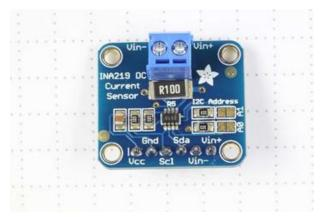
The load can be connected via the header, or using the included 2-pin screw-terminal.
