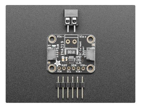
As if that weren't enough, we've now also added <u>SparkFun qwiic</u> (https://adafru.it/Fpw) compatible <u>STEMMA QT</u> (https://adafru.it/Ft4) connectors for the I2C bus so you don't even need to solder the I2C and power lines. Just wire up to your favorite micro
