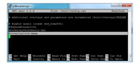
If you are using an older version of Raspberry Pi OS and there is no firmware folder, you may need to edit the /boot/config.txt file.
