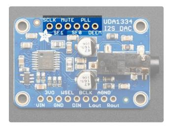
SCLK (Sys Clock) - Optional 27 MHz 'video mode' ssytem clock input - by default we generate the sysclock from the WS clock in 'audio mode' But the UDA can also take a oscillator input on this pin
