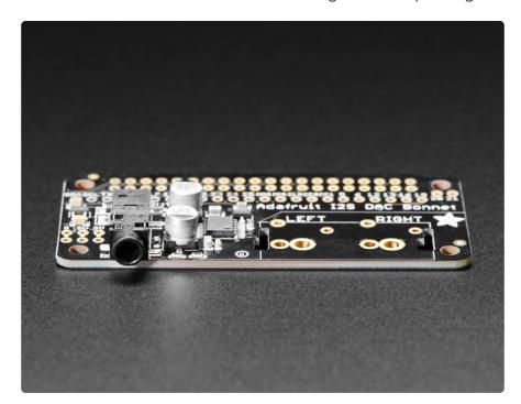
Each order comes as a fully tested and assembled PCB with a 2x20 socket connector. No soldering required! Plug it right onto your pi, install the script and reboot. Pow!
