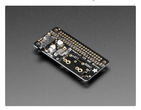
It's the exact same size as a Raspberry Pi Zero but works with **any and all** Raspberry Pi computers with a 2x20 connector - A+, B+, Zero, Pi 2, Pi 3, etc. We've tested it out with Raspbian (the official operating system) and Retropie.
