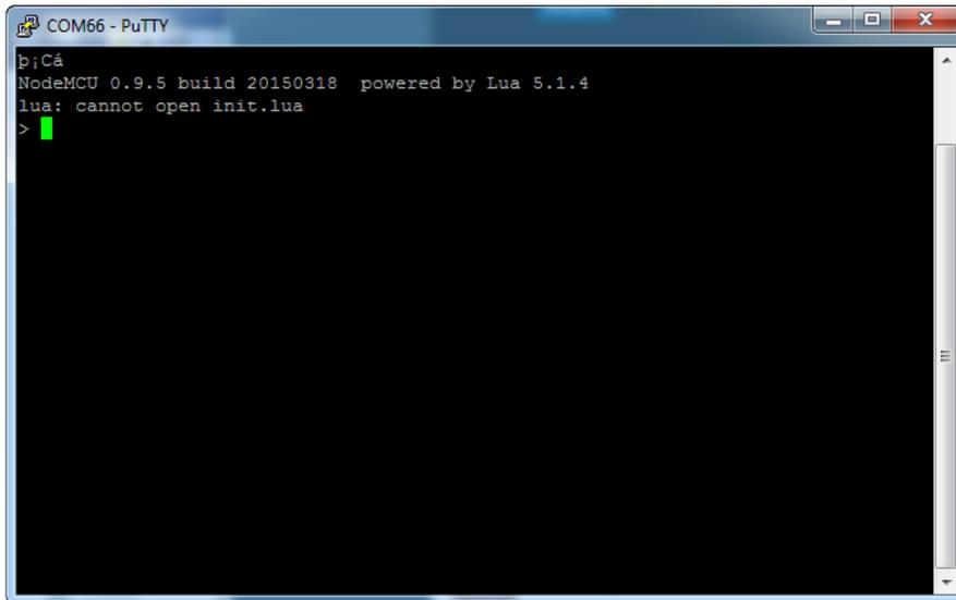
If you don't get this message, first check that the red/blue leds flickered when you press the reset button. If they didnt, make sure the board is powered via V+ or Vbat. If they do flicker, make sure you've got the right baud rate selected in the software (9600) and the RX/TX/GND pins connected right
