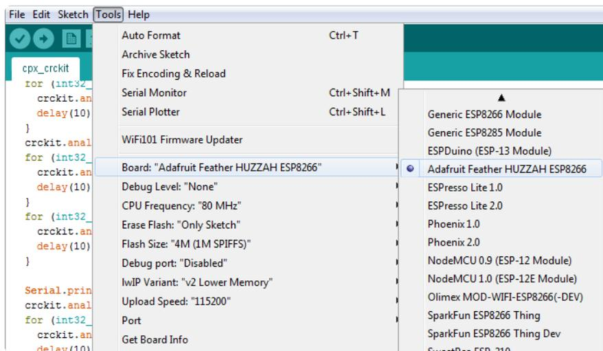
80 MHz as the CPU frequency (you can try 160 MHz overclock later)
