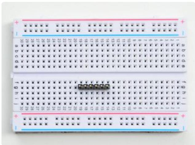
If you're planning on programming with an FTDI or console cable, it's handy to have 6 pins soldered on the end for plugging in.
