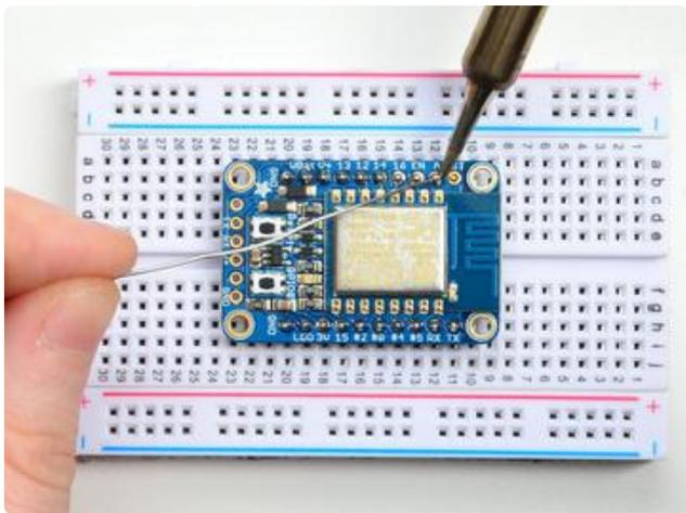
Flip the breadboard around to solder the other strip
