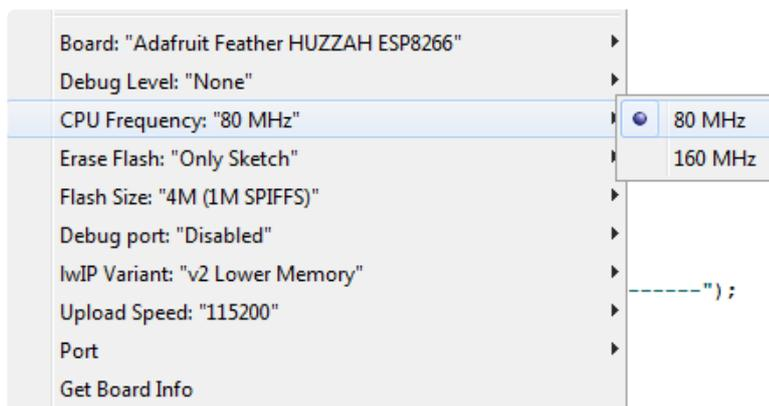
115200 baud upload speed is a good place to start - later on you can try higher speeds but 115200 is a good safe place to start. You can move down to lower speeds if you are having upload issues, or speed it up if your setup is stable, for faster uploads!
