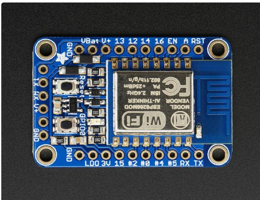
The HUZZAH ESP8266 breakout is what we designed to make working with this chip super easy and a lot of fun. We took a certified module with an onboard antenna, and plenty of pins, and soldered it onto our designed breakout PCBs. We added in:
