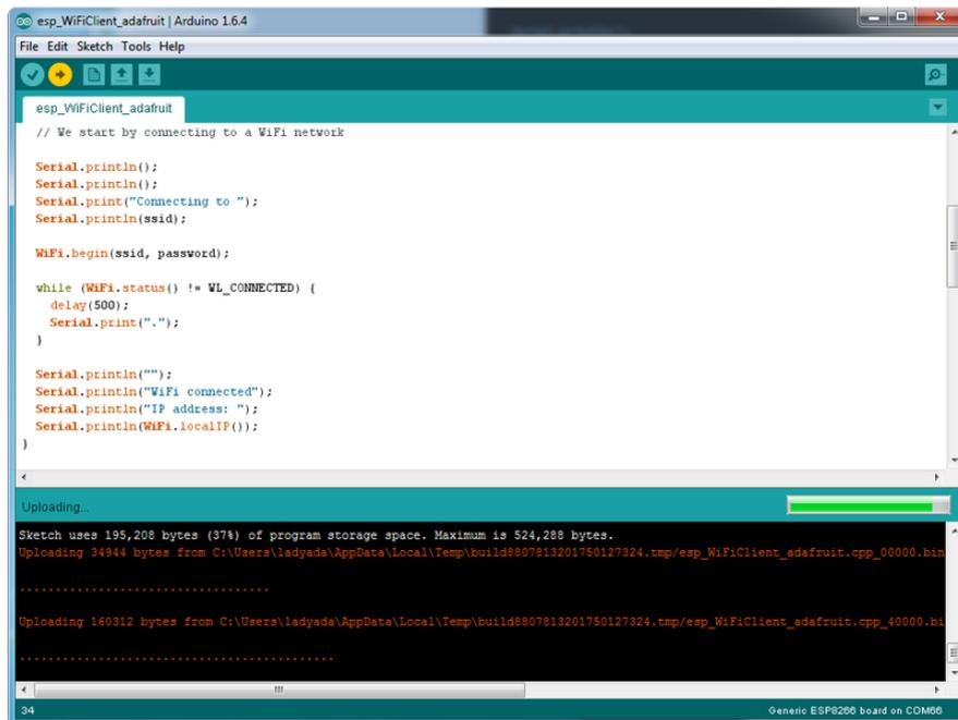
Open up the IDE serial console at 115200 baud to see the connection and webpage printout!
