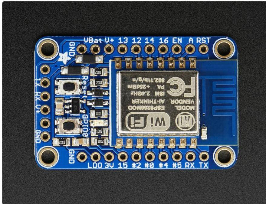
This ESP8266 breakout has a ton of pins available, compared to the mini ESP-01 module. When programming the breakout in Lua or via the Arduino IDE, you can control these I/O pins to light up LEDs, read buttons, talk to sensors etc. There's also a bunch of pins for power and control.
