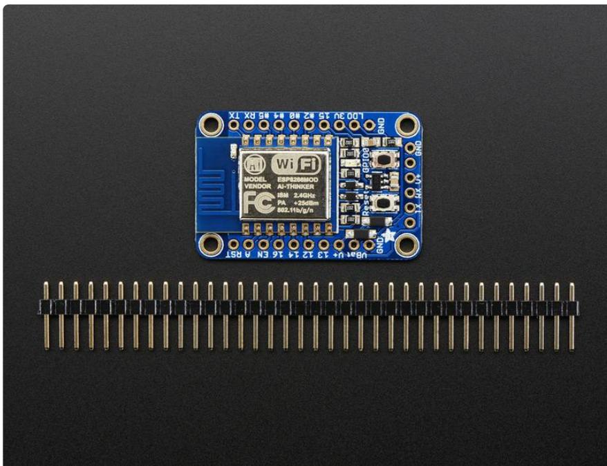
Each order comes with one assembled and tested HUZAZH ESP8266 breakout board, and a stick of 0.1" header that you can solder on and plug the breakout into a breadboard. A soldering iron and solder is required for that, and aren't included. You'll also need a USB-serial cable such as a [USB console cable \(Windows only\) \(\)](#), [FTDI Friend \(any OS\) \(http://adafruit.it/284\)](#), or [FTDI cable \(any OS\) \(http://adafruit.it/70\)](#) to upload software to the HUZAZH ESP8266!
