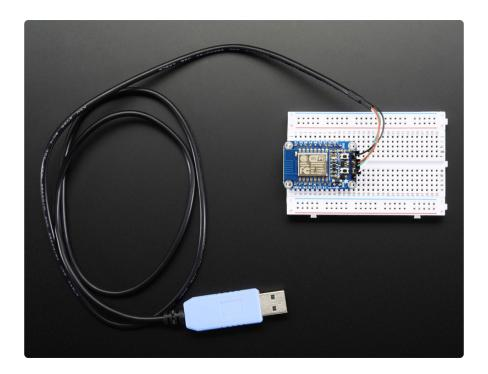
We recommend using the Arduino IDE. Once you download the ESP8266 core, you can treat it just like a microcontroller+WiFi board, no other processors needed (https://adafru.it/inB)!
