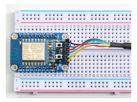
If using a console cable, connect the black wire to ground, red wire to  $\mathbf{V}+$ , white wire to  $\mathbf{T}\mathbf{X}$  and green wire to  $\mathbf{R}\mathbf{X}$
