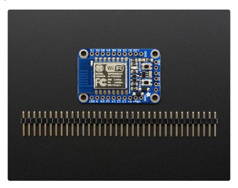
Each order comes with one assembled and tested HUZZAH ESP8266 breakout board, and a stick of 0.1" header that you can solder on and plug the breakout into a breadboard. A soldering iron and solder is required for that, and aren't included. You'll also need a USB-serial cable such as a USB console cable (Windows only) (http://adafru.it/954), FTDI Friend (any OS) (http://adafru.it/284), or FTDI cable (any OS) (http://adafru.it/70)to upload software to the HUZZAH ESP8266!
