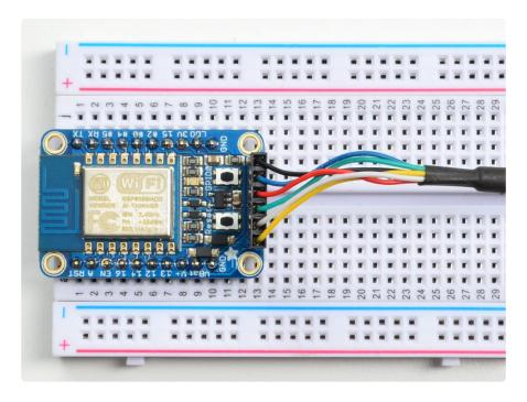
If using a console cable, connect the black wire to ground, red wire to  $\mathbf{V}^+$ , white wire to  $\mathbf{T}\mathbf{X}$  and green wire to  $\mathbf{R}\mathbf{X}$
