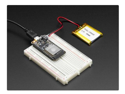
Comes fully assembled and tested, with a USB interface that lets you quickly use it with the Arduino IDE or the low-level ESP32 IDF. We also toss in some header so you can solder it in and plug into a solderless breadboard.
