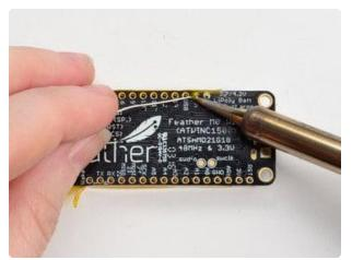
Flip & Tack Solder After flipping over, solder one or two
