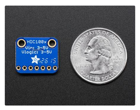
This I2C digital humidity sensor is a fairly accurate and intelligent alternative to the much simpler Humidity and Temperature Sensor - SHT15 Breakout (http://adafru.it/
