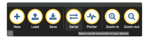
The Mu window will split in two, horizontally, and display the serial console at the bottom.
