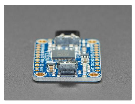
NEW: As of Feb 12, 2020 we have given this venerable board a makeover! We now have a modern USB C connector on the board (instead of micro USB), a I2C switch to
