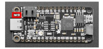
The built-in LED, indicated by the red box in the image, is labeled "13", and located above the USB Type-C connector next to the JST battery connector.
