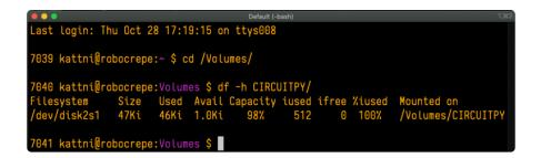
That's not very much space left! The next step is to show a list of the files currently on the CIRCUITPY drive, including the hidden files, using the **ls** command. You cannot use Finder to do this, you must do it via command line!
