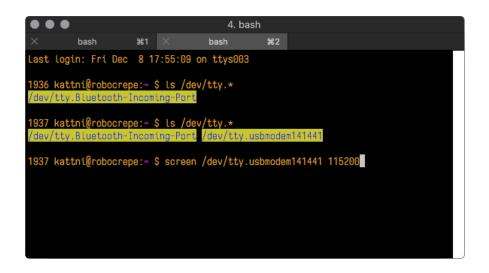
Press enter to run the command. It will open in the same window. If no code is running, the window will be blank. Otherwise, you'll see the output of your code.
