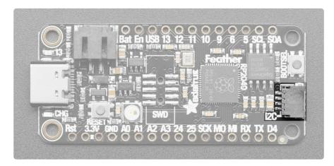
The Feather RP2040 comes with a built in STEMMA QT connector! This means you can connect up all sorts of I2C sensors and breakouts (), no soldering required! This connector uses the SCL and SDA pins for I2C, which ends up being the RP2040's I2C1 peripheral. In CircuitPython, you can use the STEMMA connector with board.SCL an d board.SDA, or board.STEMMA\_I2C(). In Arduino it is Wire.
