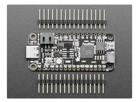
Comes fully assembled and tested, with the UF2 USB bootloader. We also toss in some header, so you can solder it in and plug it into a solderless breadboard.
