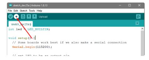
The IDE will try to compile the sketch again for good measure, then it will try to connect to the board and upload a the file.
