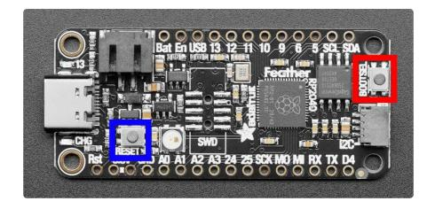
To enter the bootloader, hold down the BOOT/BOOTSEL button (highlighted in red above), and while continuing to hold it (don't let go!), press and release the reset button (highlighted in blue above). Continue to hold the BOOT/BOOTSEL button until the RPI-RP2 drive appears!
