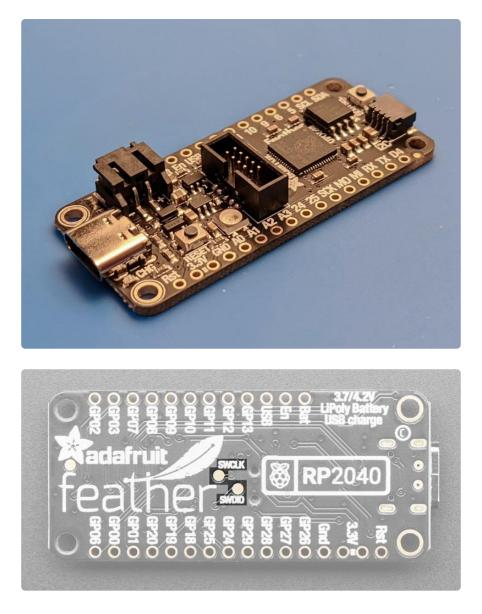
On the back of the board are pads for the SWCLK and SWDIO pins. They provide access to the internal Serial Wire Debug multi-drop bus, which provides debug access to both processors, and can be used to download code.
