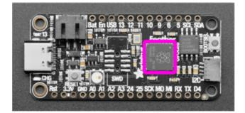
The microcontroller on the Feather RP2040 is located to the right-center of the board, nested between the Adafruit Feather RP2040 label on the silk.
