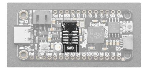
For advanced debugging or to reprogram your Feather RP2040, there is a footprint to solder a 2\*5 pin 0.05" standard SWD header on the board. The image above shows the "pin 1" location by marking it with a triangle. This orientation places the connector key facing towards the end of the board where the USB connector is. This allows you to use something like a <u>Segger J-Link</u> () and a <u>1.27mm SWD cable</u> () to connect from your PC to the Feather.
