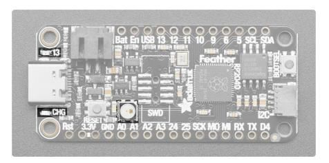
Above the pin labels for AO and A1 is the status NeoPixel LED. In CircuitPython, the NeoPixel is **board.NEOPIXEL** and the library for it is <u>here</u> () and in <u>the bundle</u> (). The NeoPixel is powered by the 3.3V power supply but that hasn't shown to make a big difference in brightness or color. In CircuitPython, the LED is used to indicate the runtime status.
