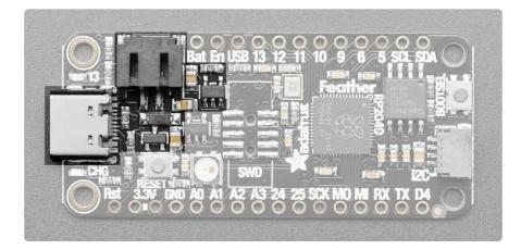
The above shows the USB-C jack (left), LiPoly JST jack (top left), as well as the changeover diode (just to the right of the JST jack) and the LiPoly charging circuitry (to the right of the JST jack).
