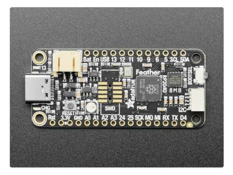
As of November 28, 2022 – we've updated this Feather with a right-angle tactile button for the Bootloader switch, so that you can press it even when a 'wing is on the Feather. We have also connected the boot button to GPIO #4 so it can be used as a user-input button.
