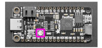
The NeoPixel LED (indicated by the magenta box in the image) is located above the A0 and A1 labels on the silk.
