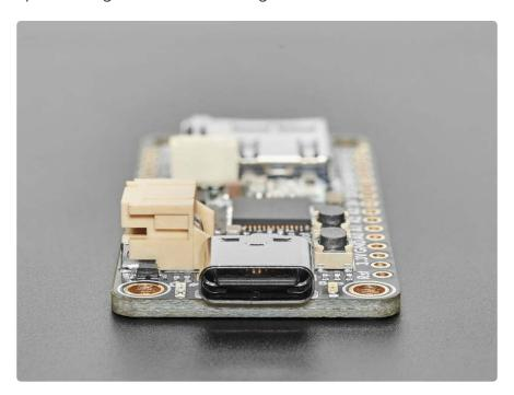
To make it easy to use for portable projects, we added a connector for any of our 3.7V Lithium polymer batteries and built-in battery charging. You don't need a battery, it will run just fine straight from the USB Type C connector. But, if you do have a battery, you
