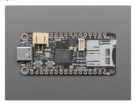
This is the Adafruit Feather RP2040 Adalogger - our take on an 'all-in-one' RP2040 data-logger (or data-reader) with built-in USB, battery charging, and a microSD holder ready to rock! We have other boards in the Feather family, check'em out here (https://adafru.it/17B).
