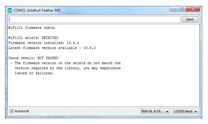
No problem - you can update the firmware through your Arduino/compatible! You must use a 1.8.x version of Arduino IDE. See the orange box below. Start by loading up the FirmwareUpdater sketch
