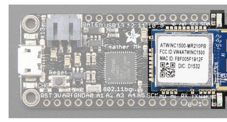
Since not all pins can be brought out to breakouts, due to the small size of the Feather, we use these to control the WiFi module
