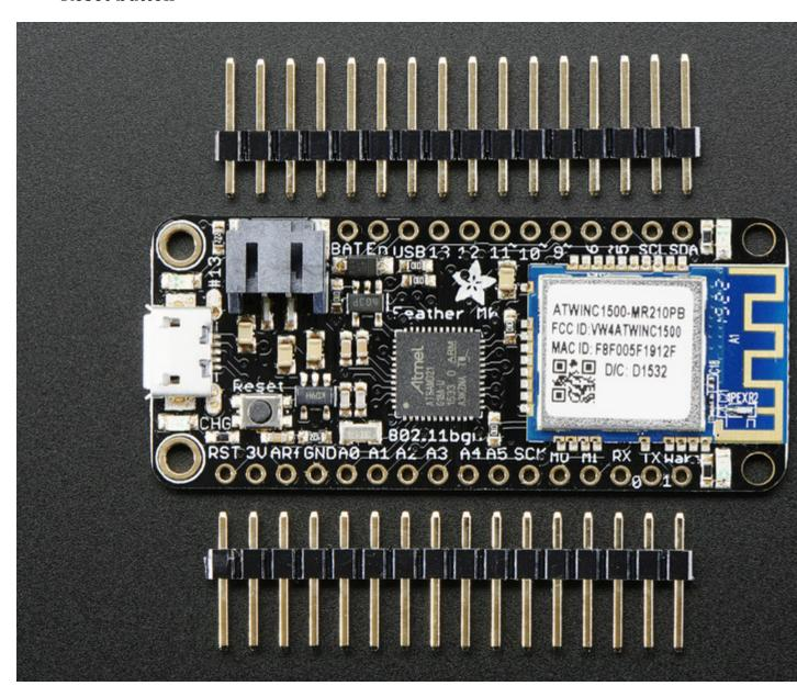
Comes fully assembled and tested, with a USB bootloader that lets you quickly use it with the Arduino IDE. We also toss in some header so you can solder it in and plug into a solderless breadboard. Lipoly battery (https://adafru.it/e0v) and MicroUSB cable (https://adafru.it/aM5) not included (but we do have lots of options in the shop if you'd like!)
