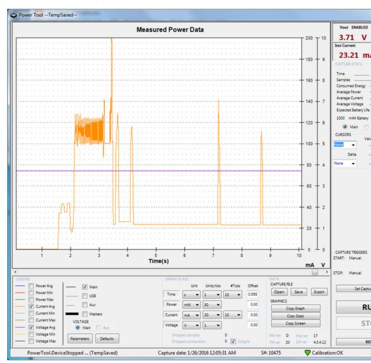
Note that 10mA or so is for the ATSAMD chip, so that means you've got ~12mA for the WiFi module.
