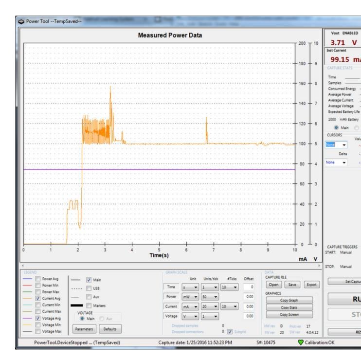
You can see the chip launch at about 1.5 seconds, then turn on the WiFi and at about 2s make the SSID connection and MQTT connection. The average current is about 100ms afterwards, and a packet spikes up to ~130mA at the 7 second mark.
