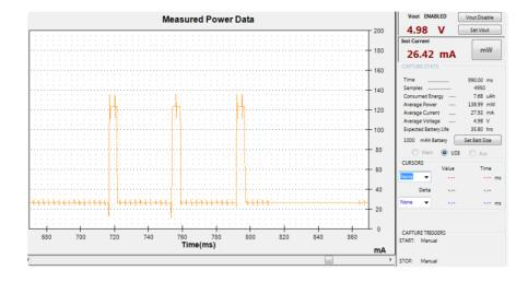
Here is a transmit with radio.setPowerLevel(0) to set +5dBm power
