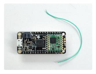
Cut a stranded or solid core wire to the proper length for the module/frequency
