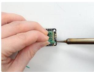
Strip a mm or two off the end of the wire, tin and solder into the ANT pad on the very right hand edge of the Feather
