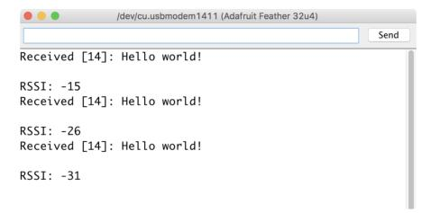
To receive a message simply call the <a href="receive">receive</a> function. This function will wait for half a second for any packet to be received. If a packet is found it will be returned as
