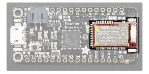
Since not all pins can be brought out to breakouts, due to the small size of the Feather, we use these to control the BLE module
