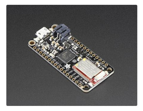
At the Feather MO's heart is an ATSAMD21G18 ARM Cortex MO processor, clocked at 48 MHz and at 3.3V logic, the same one used in the new <u>Arduino Zero</u> (http://adafru.it/2843). This chip has a whopping 256K of FLASH (8x more than the Atmega328 or 32u4) and 32K of RAM (16x as much)! This chip comes with built in USB so it has USB-to-Serial program & debug capability built in with no need for an FTDI-like chip.
