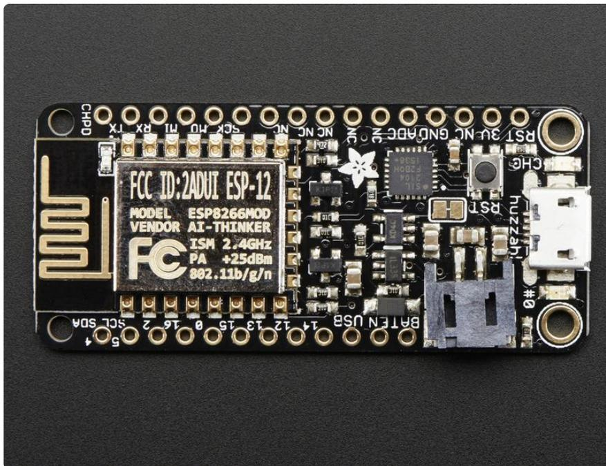
While the Feather HUZZAH ESP8266 comes pre-programmed with NodeMCU's Lua interpreter, you don't have to use it! Instead, you can use the Arduino IDE which may be more familiar. This will write directly to the firmware, erasing the NodeMCU firmware, [so if you want to go back to Lua, use the flasher to re-install it \(https://adafru.it/f1O\)](https://adafru.it/f1O)
