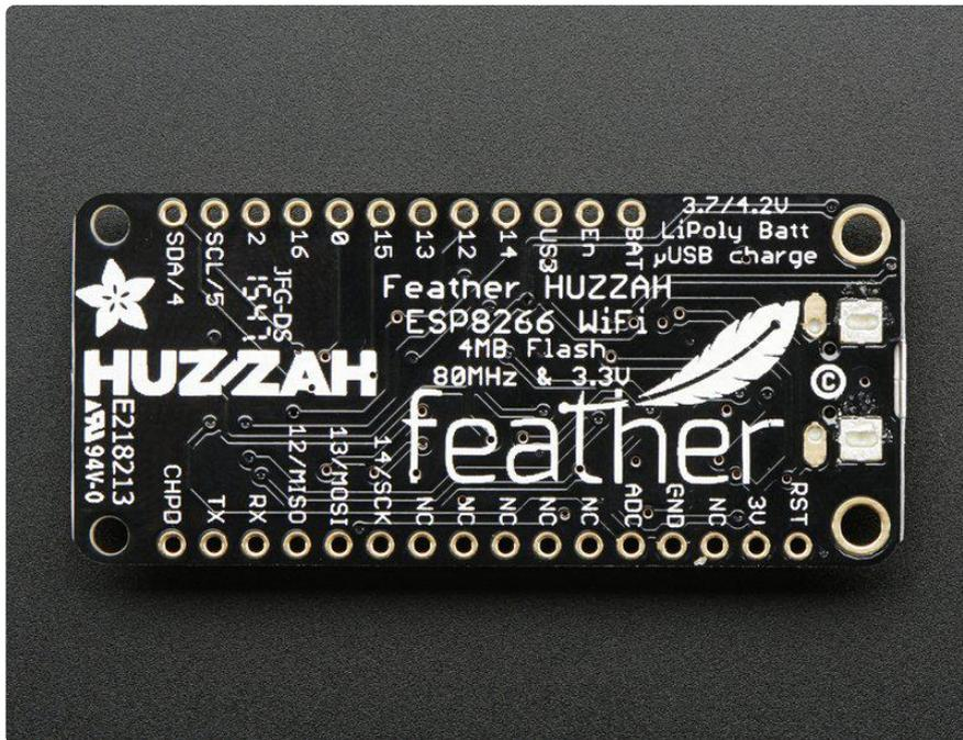
Comes fully assembled and tested, with a USB interface that lets you quickly use it with the Arduino IDE or NodeMCU Lua. (It comes preprogrammed with the Lua interpreter) We also toss in some header so you can solder it in and plug into a solderless breadboard. Lipoly battery and USB cable not included (but we do have lots of options in the shop if you'd like!)
