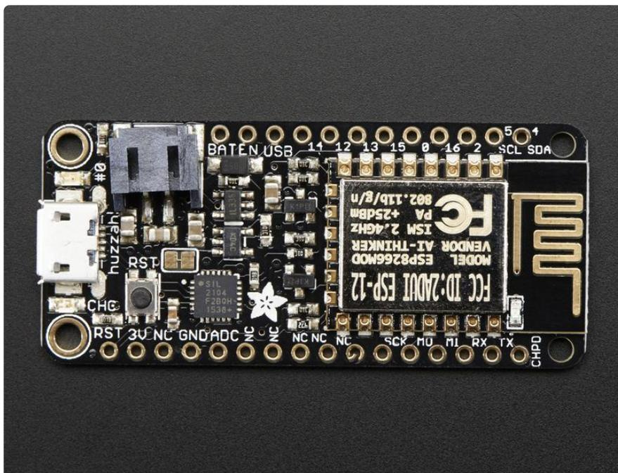
At the Feather Huzzah's heart is an ESP8266 WiFi microcontroller clocked at 80 MHz and at 3.3V logic. This microcontroller contains a Tensilica chip core as well as a full WiFi stack. You can program the microcontroller using the Arduino IDE for an easy-to-run Internet of Things core. We wired up a USB-Serial chip that can upload code at a blistering 921600 baud for fast development time. It also has auto-reset so no noodling with pins and reset button pressings.
