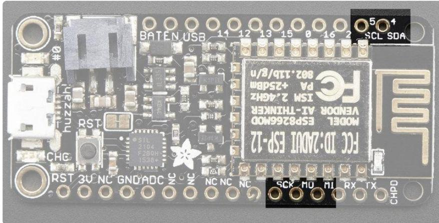
In theory you can use any pins for I2C and SPI but to make it easier for people using existing Arduino code, libraries, sketches we set up the following:
