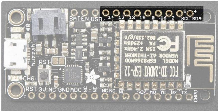
This breakout has 9 GPIO: #0, #2, #4, #5, #12, #13, #14, #15, #16 arranged at the top edge of the Feather PCB
