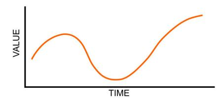
Analog signals are continuous values which means they can be an infinite number of different voltages. Think of analog signals like a floating point or fractional number, they can smoothly transiting to any in-between value like 1.8V, 1.81V, 1.801V, 1.8001V, 1.80001V and so forth to infinity.
