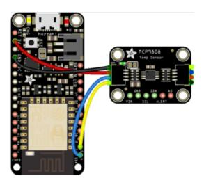
If you're using a breadboard or a "STEMMA QT / Qwiic JST SH 4-pin to Premium Male Headers Cable":
