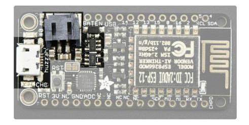
The above shows the Micro USB jack (left), LiPoly JST jack (top left), as well as the 3.3V regulator and changeover diode (just to the right of the JST jack) and the LiPoly charging circuitry (right below the regulator).
