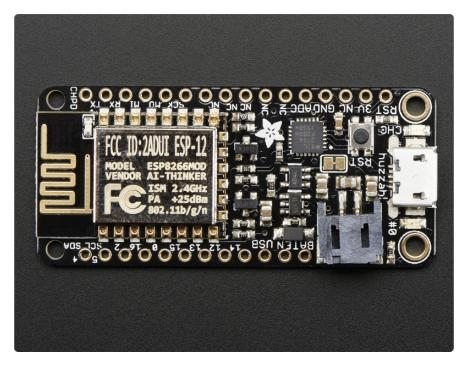
While the Feather HUZZAH ESP8266 comes pre-programmed with NodeMCU's Lua interpretter, you don't have to use it! Instead, you can use the Arduino IDE which may be more familiar. This will write directly to the firmware, erasing the NodeMCU firmware, so if you want to go back to Lua, use the flasher to re-install it (https://adafru.it/f1O)
