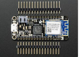
The first option is soldering in plain male headers, this lets you plug in the Feather into a solderless breadboard
