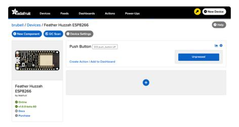
Push the button on your board to change the value of the push-button component on Adafruit IO.
