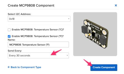
The board page should now show the MCP9808 component you created. After the interval you configured elapses, the WipperSnapper firmware running on your board automatically reads values from the sensor and sends them to Adafruit IO.
