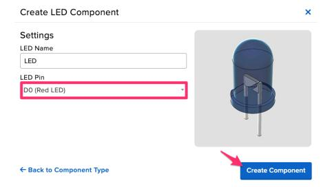
Behind the scenes, Adafruit IO sends send a command to your board running WipperSnapper telling it to configure "LED Pin" as a digital output.
