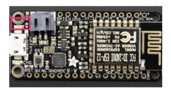
The Adafruit Feather HUZZAH ESP8266 has a LED (highlighted in red and labeled on the silkscreen as #0) above the Micro-USB port.
