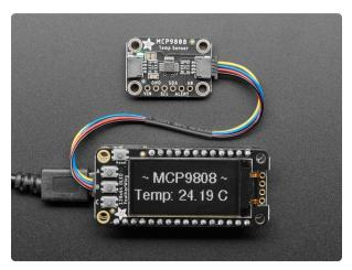
Adafruit MCP9808 High Accuracy I2C Temperature Sensor Breakout
