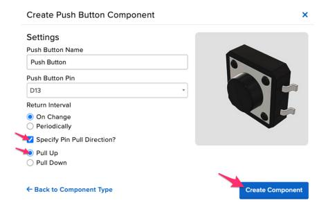
Adafruit IO sends a command to your WipperSnapper board, telling it to configure the GPIO pin you selected to behave as a digital input pin and to enable it to pull up the internal resistor.
