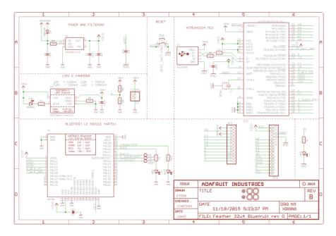
We've changed the regulator from an SPX3819 to AP2112 - it has lower dropout but cannot handle higher than 6V
