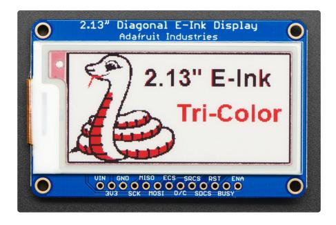
This e-Paper display uses SPI to receive image data. Since the display is SPI, it was easy to add two more SPI devices to share the bus - an SPI SRAM chip and SPI-driven
