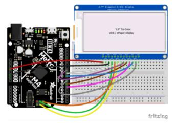
Vin connects to the microcontroller board's 5V or 3.3V power supply pin GND connects to ground CLK connects to SPI clock. It's easiest to connect it to pin 3 of the ICSP header. MOSI connects to SPI MOSI. It's easiest to connect it to pin 4 of the ICSP header. MISO connects to SPI MISO. It's easiest to connect it to pin 1 of the ICSP header.
