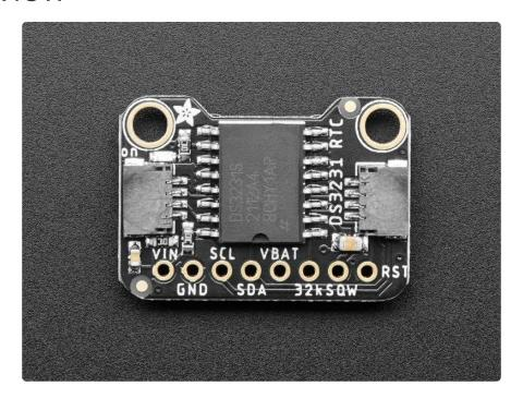
The datasheet for the DS3231 explains that this part is an "Extremely Accurate I<sup>2</sup>C-Integrated RTC/TCXO/Crystal". And, hey, it does exactly what it says on the tin! This Real Time Clock (RTC) is the most precise you can get in a small, low power package.
