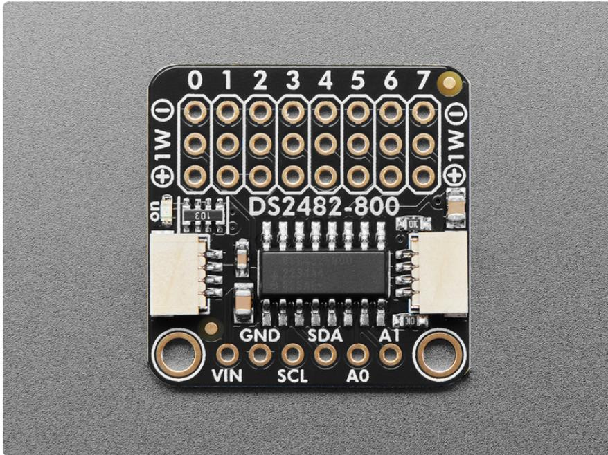
The [DS2482S-800](https://adafru.it/1a7j) (<https://adafru.it/1a7j>) is a Stemma QT board that uses a I2C-to-1Wire controller chip, with 8 selectable channels, built-in parasitic-power-pullups, adjustable I2C address and a wide operating voltage range! You can easily connect it to an existing I2C bus and then use the breakout pads to attach multiple DS18B20's, or pair it with our [1-Wire chaining breakouts](http://adafru.it/5971) (<http://adafru.it/5971>) for fancier experimentation.
