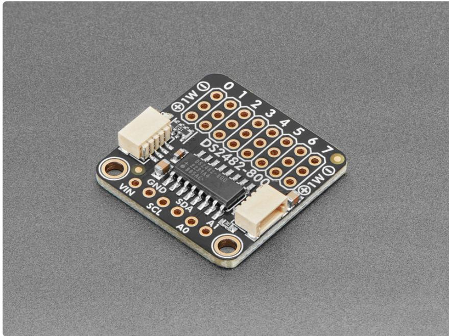
To get you going fast, we spun up a custom-made PCB in the [STEMMA QT form factor](https://adafru.it/LBQ) (<https://adafru.it/LBQ>), making it easy to interface. The [STEMMA QT connectors](https://adafru.it/JqB) (<https://adafru.it/JqB>) on either side are compatible with the [SparkFun Qwiic](https://adafru.it/Fpw) (<https://adafru.it/Fpw>) I2C connectors.
