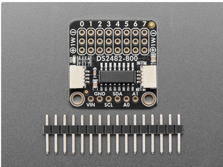
You might be wondering: if you can connect multiple 1-Wire devices on a single wire, then why have 8 channels on this breakout? Reason is: if you have 8 temperature sensors, there's no easy way to know which one is which other than connecting them one at a time and reading the unique ROM identifier. With this breakout you can select the channel so you know for sure which location is being measured, even if the sensor is swapped out later.
