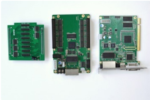
From left to right: IDC adapter for the receiver, receiver card, & sender card.
