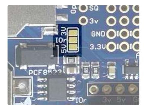
The IOREF pin should come from the Arduino main board being used.
