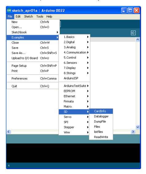
This sketch will not write any data to the card, just tell you if it managed to recognize it, and some information about it. This can be very useful when trying to figure out whether an SD card is supported. Before trying out a new card, please try out this sketch!
