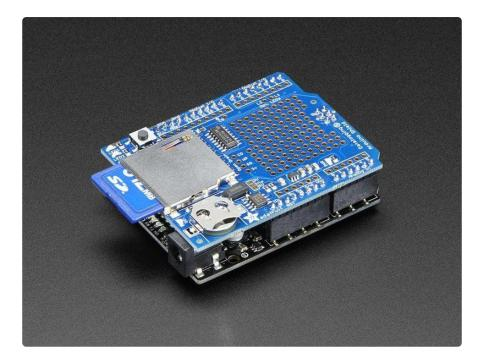
Here's a handy Arduino shield: we've had a lot of people looking for a dedicated and well-designed data logging shield. We worked hard to engineer an inexpensive but well-rounded design. This shield makes it easy to add a 'hard disk' with gigabytes of storage to your Arduino!
