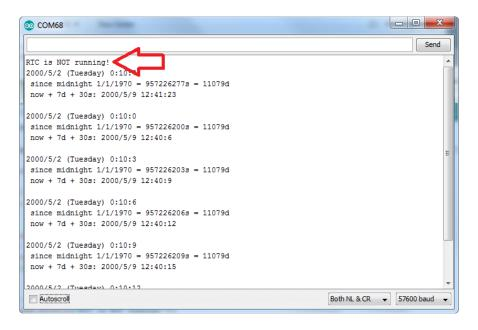
Whenever the RTC chip loses all power (including the backup battery) it will reset to an earlier date and report the time as 0:0:0 or similar. The DS1307 won't even count seconds (it's stopped). Whenever you set the time, this will kickstart the clock ticking.
