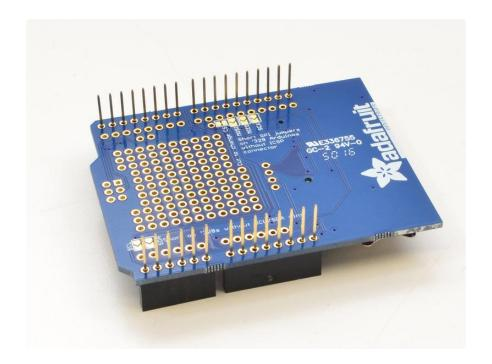
Be sure to insert the headers from the TOP of the shield so that they can be soldered from the BOTTOM.
