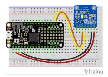
Board 3V to sensor VIN Board GND to sensor GND Board SCL to sensor SCL Board SDA to sensor SDA
