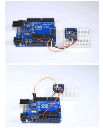
Arduino Wiring: Connect jumpers from: 5v -> VIN (red wire) GND -> GND (black wire) SDA -> SDA (orange wire) SCL -> SCL (white wire) Note: On older Arduinos such as the Duemilanove and pre R3 UNOs, SDA is on Analog 4 and SCL is on Analog 5.
