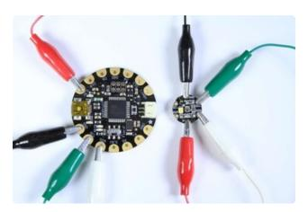
Flora Wiring: Connect from: 3.3v -> 3v (red wire) GND -> GND (black wire) SDA -> SDA (white wire) SCL -> SCL (green wire)
