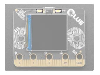
Bright white LEDs - On the front of the board are two bright white LEDs for illumination and color sensing.
