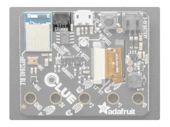
Qwiic / STEMMA QT connector -Use to add more sensors, motor controllers, or displays over I2C.
