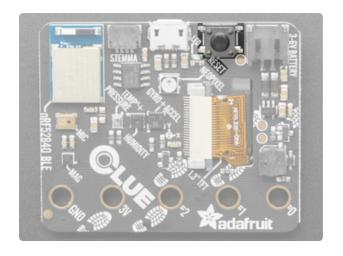
Reset button - This button resets the board. Press once to reset.
