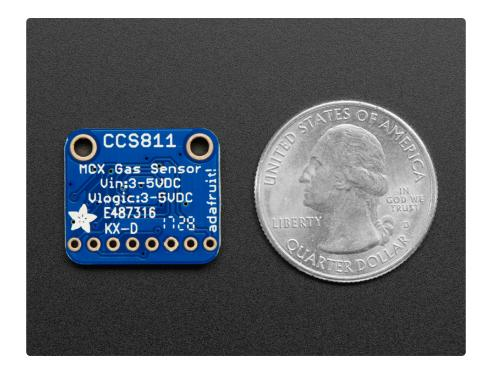
The CCS811 has a 'standard' hot-plate MOX sensor, as well as a small microcontroller that controls power to the plate, reads the analog voltage, and provides an I2C interface to read from.
