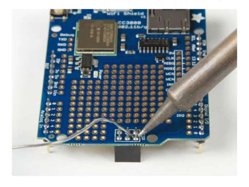
By default, SPI through the ICSP header is not connected. To enable the ICSP header connections, you'll have to connect three solder jumpers on the bottom of the
