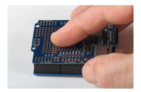
Place the shield over the pins, and carefully solder each one in place (see our <u>Guide</u> <u>To Excellent Soldering</u> (https://adafru.it/aTk) for instructions and tips on getting the best results).
