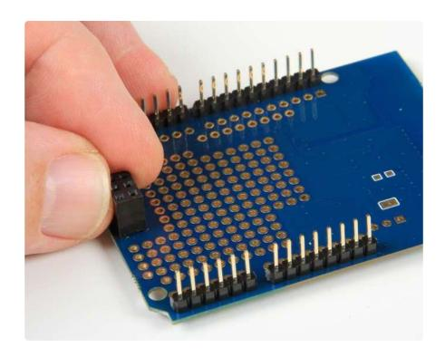
The shield also comes with a 2X3 pin female header socket. This will plug into the 2X3 ICSP pin header on your Arduino, to bring SPI up to the shield. This allows you to use the shield with an Arduino Mega, Leonardo, or Due without having to cut traces or solder jumper wires for SPI.
