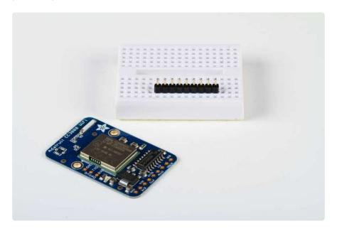
Set the breakout board over the pins, and carefully solder each pin (see our <u>Guide To Excellent Soldering</u> (https://adafru.it/aTk) for instructions and tips on getting the best results).
