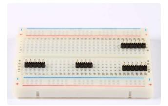
Position the header strips Plug them long-pins down into a breadboard to stabilize them for soldering.
