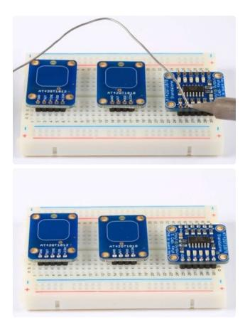
And Solder Solder each pin for solid electrical contact.
