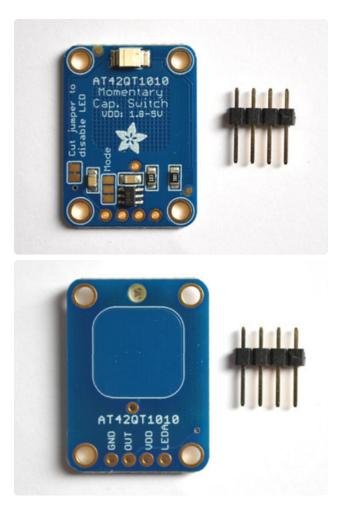
Momentary This sensor has a built-in sense-pad and is active for as long as the sensor area is touched.
