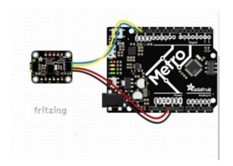
To connect the assembled BNO055 breakout to an Arduino Uno, follow the wiring diagram.
