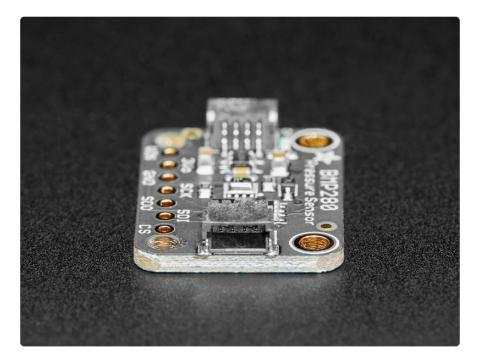
Nice sensor right? So we made it easy for you to get right into your next project. The surface-mount sensor is soldered onto a custom made PCB in the <u>STEMMA QT form</u> factor (https://adafru.it/LBQ), making them easy to interface with. The <u>STEMMA QT</u> connectors (https://adafru.it/JqB) on either side are compatible with the <u>SparkFun</u> Qwiic (https://adafru.it/Fpw) I2C connectors. This allows you to make solderless
