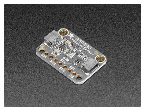
Bosch has stepped up their game with their new BMP280 sensor, an environmental sensor with temperature, barometric pressure that is the next generation upgrade to the BMP085/BMP180/BMP183. This sensor is great for all sorts of weather sensing and can even be used in both I2C and SPI!
