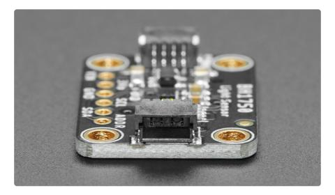
To make things easier and a bit more flexible, we've also included SparkFun Qwiic () compatible STEMMA QT () connectors for the I2C bus so you don't even need to solder! Just plug in a compatible cable and attach it to your MCU of choice and you're ready to load up some software and measure some light. To help with the software
