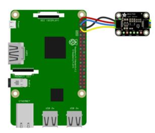
Pi 3V to sensor VCC (red wire)
