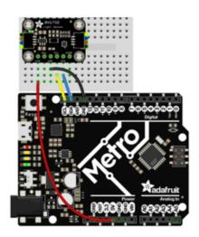
Connect board VIN (red wire) to Arduino 5V if you are running a 5V board Arduino (Uno, etc.). If your board is 3V, connect to that instead.
