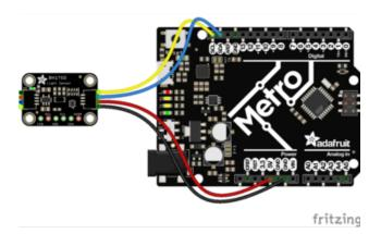
Connect board VIN (red wire) to Arduino 5V if you are running a 5V board Arduino (Uno, etc.). If your board is 3V, connect to that instead.
