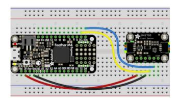
Board 3V to sensor VIN (red wire)
