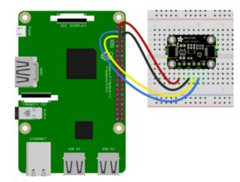
Pi 3V to sensor VCC (red wire)
