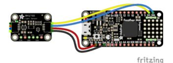
Board 3V to sensor VIN (red wire)
