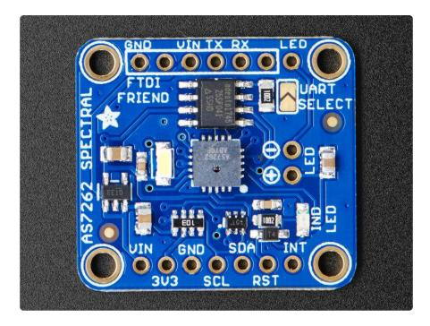
This sensor has 4 mounting holes and 2 header breakout strips.
