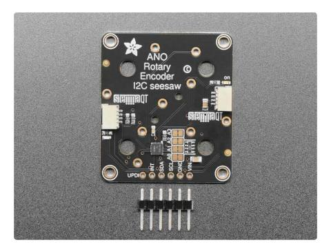
The ANO rotary encoder wheel is a funky user interface element, reminiscent of the original clicking scroll wheel interface on the first iPods (). It's a nifty kit, but the pin-out is a little odd - and there are a ton of pins needed to connect to the rotary encoder and 5 button switches.
