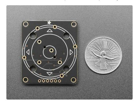
Four solder jumpers can be used to change the I2C address - up to 16 can share one I2C bus! If you happen to need more, it's possible to set the I2C address with a
