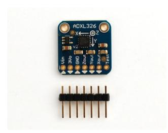
The ADXL326 can measure at least +/16G(!) in the X, Y and Z axis. It is ideal for measuring more dynamic accelerations from high-performance land and air vehicles as well as for shock and impact measurements.
