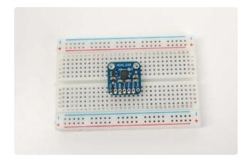
Add the breakout board: Place the breakout board over the pins.
