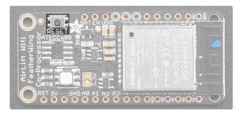
Tap this button twice to enter the bootloader. If it doesn't work on the first try, don't be discouraged. The rhythm of the taps needs to be correct and sometimes it takes a few tries.
