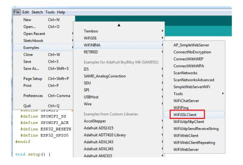
Note we use WiFiSSLClient client; instead of WiFiClient client; to require an SSL connection!
