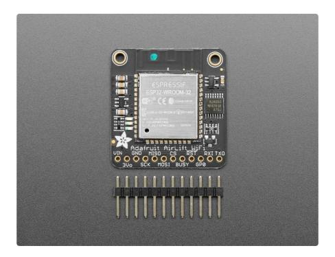
The ESP32 also supports BLE (Bluetooth Low Energy), though not simultaneously with WiFi. Many of our CircuitPython builds include native support for ESP32 BLE. You use a few control pins and the RXI and TXO pins to talk to the ESP32 when it's in BLE mode.
