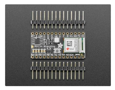
We placed an ESP32 module on a BitsyWing with a tri-state chip for MOSI so you can share the SPI bus. The add on comes fully assembled and tested, pre-programmed with ESP32 SPI WiFi co-processor firmware that you can use in CircuitPython to use this into WiFi co-processor over SPI + 2 pins (https://adafru.it/EvI). We also toss in some header so you can solder it in though you'll need stacking headers for your ItsyBitsy to put the add-on on top.
