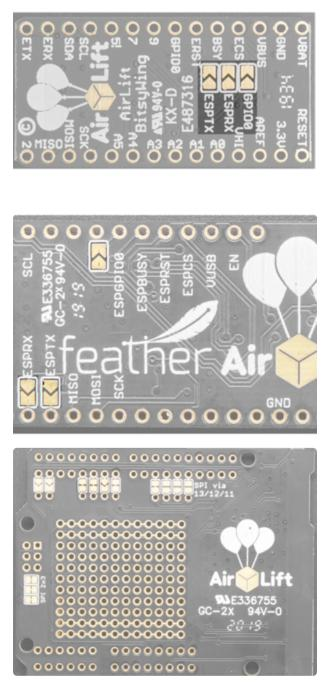
Make sure to solder each of these pads together. You will not be able to upload firmware to your ESP32 if they are not connected.
