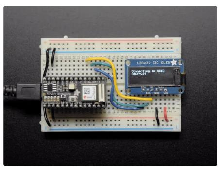
The antenna on the new, smaller ESP32 module is very delicate! Avoid touching it and grab the add-on by the long sides to avoid smushing the antenna
