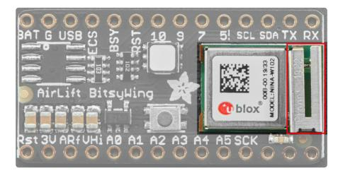
To stack the Airlift Add-on on top of the ItsyBitsy, you'll need stacking headers for the ItsyBitsy. For now you'll need to cut down a set of Feather Stacking Headers (https://adafru.it/oAP) to fit the ItsyBitsy however we will have headers with the correctly length soon!
