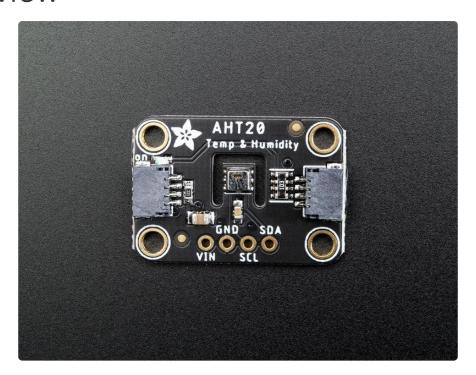
The AHT20 is a nice but inexpensive temperature and humidity sensor <u>from the same</u> <u>folks that brought us the DHT22</u> (https://adafru.it/sb4). You can take sensor readings as often as you like, and it uses standard I2C so its super easy to use with any Arduino or Linux/Raspberry Pi board.
