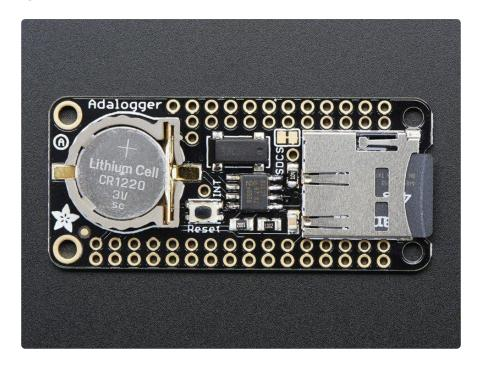
A Feather board without ambition is a Feather board without FeatherWings! This is the Adalogger FeatherWing: it adds both a battery-backed Real Time Clock and micro SD card storage to any Feather main board. Using our Feather Stacking Headers (htt p://adafru.it/2830) or Feather Female Headers (http://adafru.it/2886) you can connect a FeatherWing on top of your Feather board and let the board take flight!
