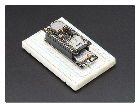
But don't forget, you can also put the stacking headers on the wing and stack the Feather on top of it!
