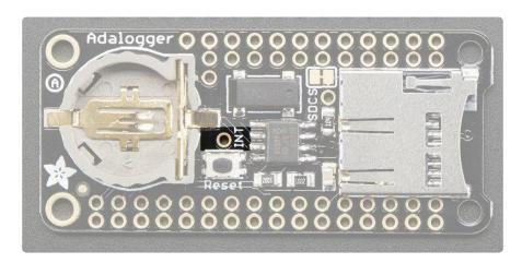
There's also a breakout for INT which is the output pin from the RTC. It can be used as an interrupt output or it could also be used to generate a square wave.
