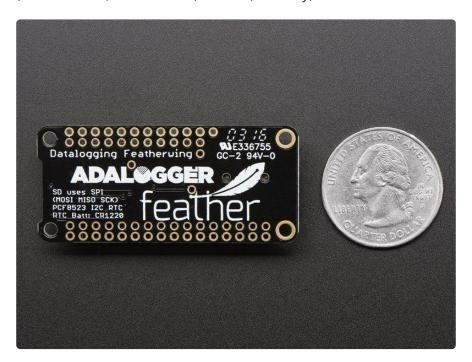
We recommend the Arduino's default SD library to talk to the microSD card socket. On ESP8266, the SD CS pin is on GPIO 15, on Atmel M0, M4, 328P or 32u4 it's on GPIO 10. You can cut the trace to the default pin and change this to any pin. To use the RTC, use our RTClib library (https://adafru.it/c7r). If you need a precision RTC, check out our DS3231 FeatherWing (http://adafru.it/3028)
