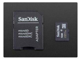
4GB Blank SD/MicroSD Memory Card Add mega-storage in a jiffy using this 4 GB micro-SD card. It comes with a SD adapter so you can use it with any of our shields or adapters! Preformatted to FAT so it works out of...
