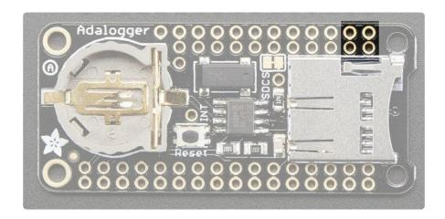
In the top right, SDA (rightmost) and SCL (to the left of SDA) are used to talk to the RTC chip.
