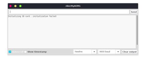
It couldn't even initialize the SD card. This can also happen if there's a soldering error or if the card is really damaged
