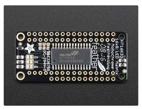
The 16x8 backpack is also great for making scrolling displays or small video displays. In our example, we set it up to display small bitmap emoticons but you can also display text that moves - kind of like a sign in front of a miniature car dealership.
