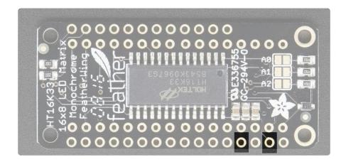
The LED matrix uses only the 3V and GND pins for power and logic. Current draw depends on how many LEDs are lit but you can approximate it as about 120mA for most uses.
