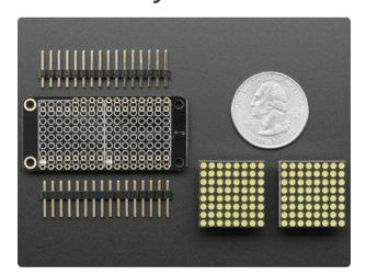
When you buy a pack from Adafruit, it comes with the fully tested and assembled backpack as well as a two 8x8 dual displays in one of the colors we provide (say, red, yellow, blue or green). You'll need to solder the matrix onto the backpack but it's an easy task.
