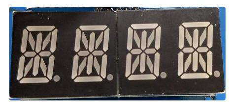
To access the individual digits, it's the same as with the 7-segment display. However, the 14-segment display can take any alphanumeric character. For example:
