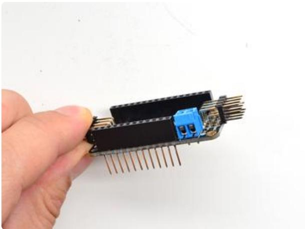
Next we will solder in the right angle header blocks used to plug in servos into the FeatherWing. There are two blocks, each are 3x4 headers in size.
