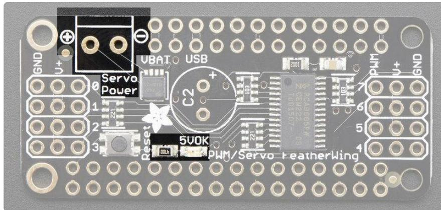
When the servo power pin is powered, the 5VOK LED will be lit. If this LED is not lit, the V+ pins will not have any voltage on them and the servos won't be powered.
