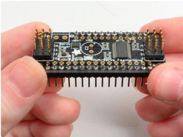
Next we will solder in the larger header blocks used to plug in servos into the FeatherWing. There are two block, each are 3x4 headers in size.
