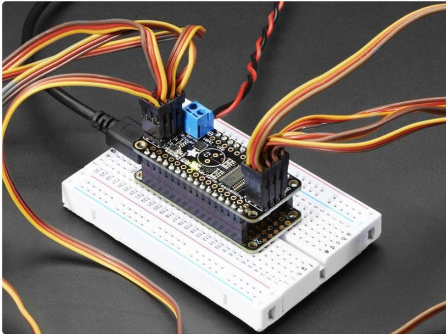
Since the FeatherWing only uses the I2C (SDA & SCL pins), it works with any and all Feathers- ATmega32u4, ATSAM M0 or ESP8266-based. You can stack it with any other FeatherWing or with itself (just make sure you have each wing with a unique I2C address) [Check out our range of Feather boards here. \(https://adafru.it/l7B\)](https://adafru.it/l7B)
