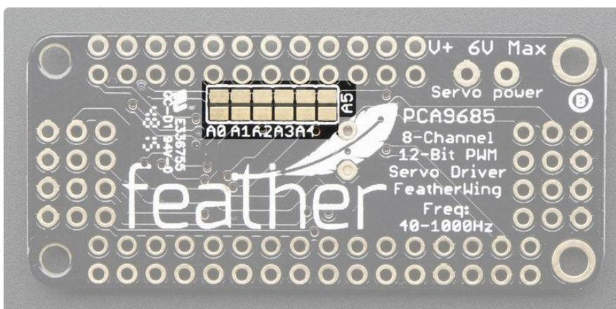
To program the address offset, use a drop of solder to bridge the corresponding address jumper for each binary '1' in the address.
