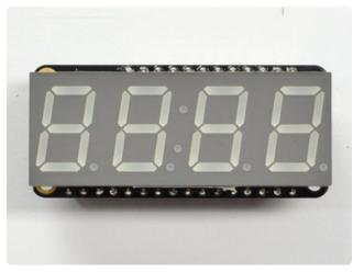
Slot the LED module on top, check again that you have it right way up!
