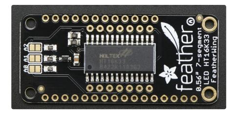
The 7-segment backpack makes it really easy to add a 4-digit numeric display with decimal points and even 'second colon dots' for making a clock
