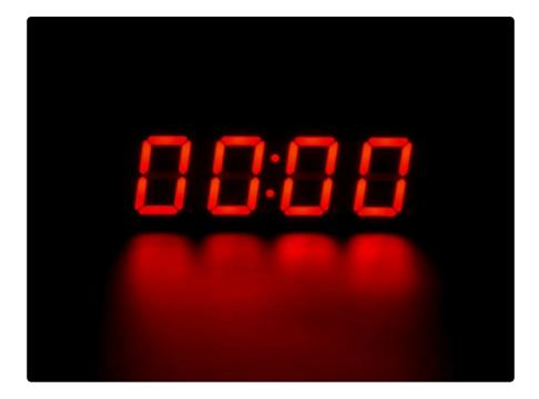
The LEDs themselves do not connect to the Feather. Instead, a matrix driver chip (HT16K33) does the multiplexing for you. The Feather simply sends i2c commands to the chip to tell it what LEDs to light up and it is handled for you. This takes a lot of the work and pin-requirements off the Feather. Since it uses only I2C for control, it works with any Feather and can share the I2C pins for other sensors or displays.
