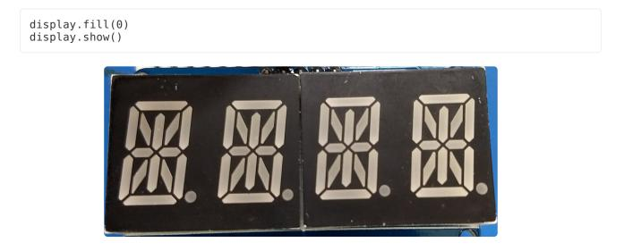
To access the individual digits, it's the same as with the 7-segment display. However, the 14-segment display can take any alphanumeric character. For example:
