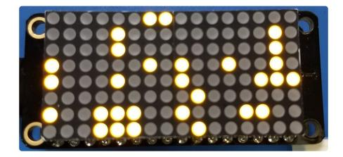
The above command will create the matrix class using the default I2C address of the display (0x70). If you've changed the I2C address (like when using multiple
