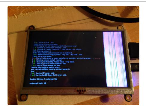
It is not broken - what is happening is you are sending 640x480 data to the monitor but since it does not have a scaler, and the display is 800x480, the remaining 160 pixels are 'not drawn' - you must set the resolution of your computer to 800x480 to
