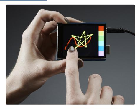
This shield uses the SPI port for sending data to the ILI9341 chipset display, and I2C for reading the TSC2007 resistive touch screen driver. That makes it work great with just about any board that is 'Arduino or Mega shaped' as long as they have the I2C SDA and SCL pins after pin D13, and the SPI 2x3 port. If you want to access the remaining pins, we recommend a WingShield (http://adafru.it/196).
