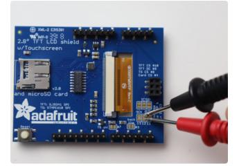
Next, take a multimeter set to the continuity setting and test that the traces were successfully separated.
