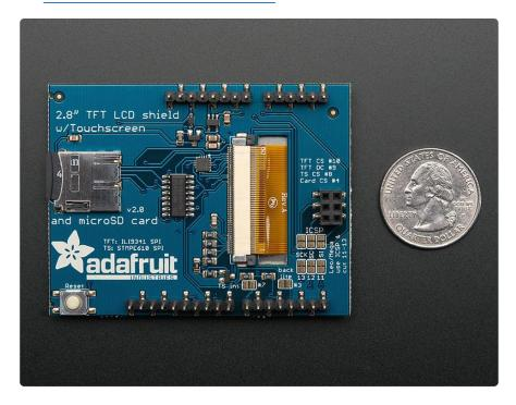
The shield is fully assembled, tested and ready to go. No wiring, no soldering! Simply plug it in and load up our library - you'll have it running in under 10 minutes! Works best with Adafruit Metro and classic Arduino (UNO, Duemilanove, Diecimila). Solder three jumpers and you can use it at full speed on an Arduino Leonardo or Mega as well.
