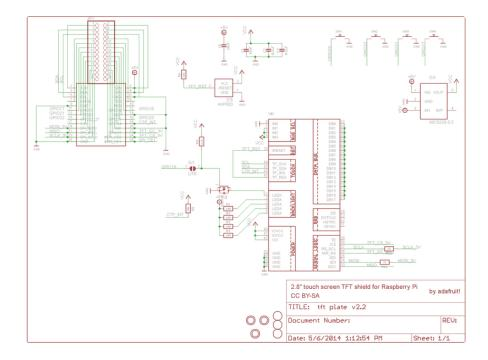
Schematic for PiTFT Plus (B+/Pi 2 shape)
