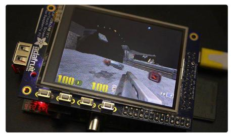
The Ideal: Adafruit's PiTFT displays are razor sharp. Whereas small composite screens on the Raspberry Pi usually require some video scaling (resulting in blurriness), PiTFT uses the GPIO header, digitally controlled pixel-by-pixel for a rock steady image. Though not a lot of pixels, it works great for retro gaming (and the display neatly stacks above the board, no side protuberances for video cables).
