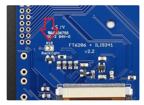
OK now you can use the PWM output on GPIO 18. There's python code available for controlling the PWM pin but you can also just use the WiringPi shell commands.
