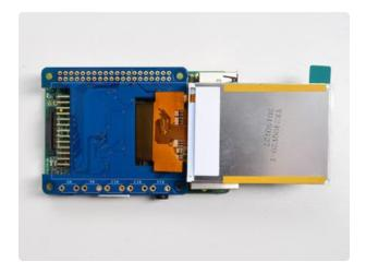
Place the PiTFT HAT on top so all the pins stick through the connector on the side. Gently flip the TFT so its off to the side and wont be in your way while you solder
