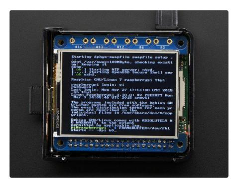
We have a right-angle 26-pin connector off to the side. You can connect a classic 26-pin Raspberry Pi GPIO cable in order to access the rest of the GPIO through a Cobbler, etc.
