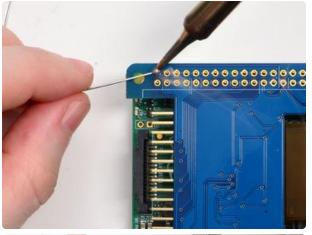
Heat up your soldering iron, and grab some solder. Start by tack-soldering one of the corners. Then you can re-heat that solder point and adjust the circuit board to make it sit flat.
