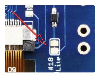
If you'd like to not have #18 control the backlight, simply cut the solder jumper, the tiny trace between the two large gold pads marked Lite #18
