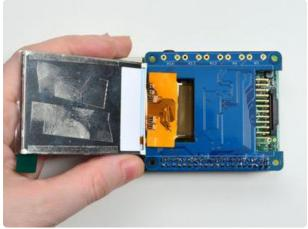
Line up the TFT screen so it matches the white outline and press it down to stick it to the circuit board
