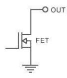
Since there is no internal connection to VCC, the open drain output does not put out a voltage like an Arduino GPIO pin. You have to provide your own external pullup. While this may seem inconvenient, the open drain configuration allows for a lot of flexibility. Since the output voltage is not dependent on the operating voltage of the breakout, you can use a variety of power sources. The FETs in the DS2413 are capable of switching voltages up to 28v and up to 20mA.
