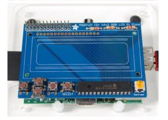
Now we will solder all 26 pins for the plate - this will send power and data between the two boards and also provide a mechanical stability. You may need to hold the plate down with tape to get it sitting flat against the Pi.
