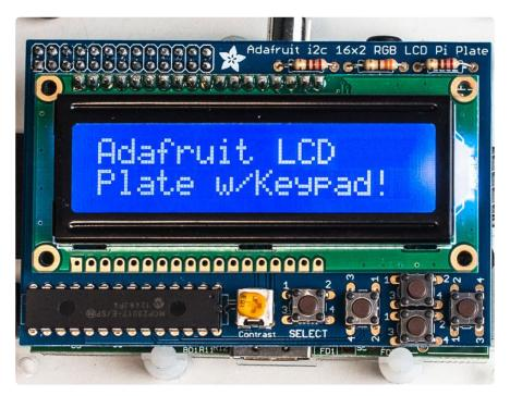
WARNING: The new Raspberry Pi model B+ with 4 USB ports overlaps closely with backlight resistor leads on the char LCD plate. You will need to cover the USB port and back of resistors with electrical tape to protect them from touching. See more details and pictures on the assembly page of this guide.
