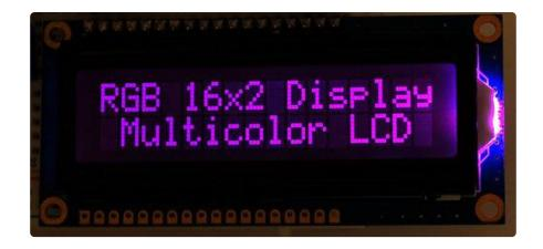
You can also use 16x2 LCDs that are the same size that do not have an RGB backlight, or have no backlight at all.
