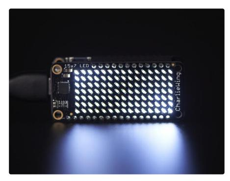
The IS31FL3731 is a nice little chip - and it runs happily over 3.3V power. Inside is enough RAM for 8 separate frames of display memory so you can set up multiple frames of an animation and flip them to be displayed with a single command. Since it uses I2C, it takes up only the SDA/SCL pins on your Feather and can share those pins with other I2C devices and sensors.
