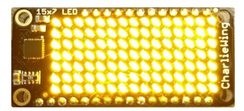
You might notice some buzzing or ringing sounds from the display when all pixels are lit, this is normal as the Charlieplex driver quickly switches LEDs on and off.
