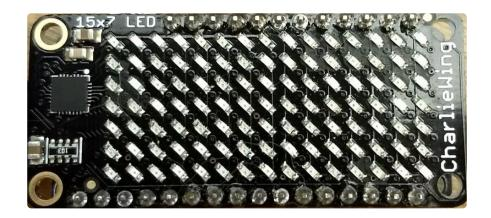
Be careful setting all pixels to 255 maximum brightness! This might pull more power than your computer's USB port can provide if you are powering your board over USB. Use an external powers supply or battery when lighting lots of LEDs to max brightness.
