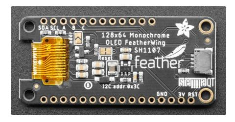
The OLED FeatherWing plugs into any Feather and adds a cute little display. To make it as cross-platform compatible as possible, we use only I2C to control the display. This is not as fast as SPI but it uses only two pins, can share the I2C bus and is fine for the small 128x62 pixel OLED.
