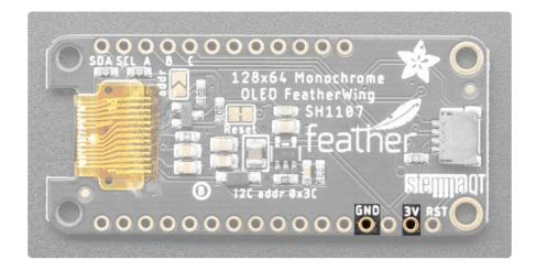
OLED displays do not have a backlight, and are fairly low power, this display will draw about 10mA when in use. The display uses 3V power and logic so we just connect to the 3V and GND pins from the feather, as indicated above.
