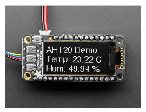
The display uses only I2C so you can easily connect it up with just two pins used (plus power and ground!). There's an auto-reset circuit and a reset button on the top. We've even included a <a href="SparkFun qwiic">SparkFun qwiic</a> (https://adafru.it/Fpw)-compatible <a href="STEMMA QT">STEMMA QT</a> (https://adafru.it/Ft4) connector for the I2C bus so you can plug and play any of our STEMMA QT, qwiic or Grove I2C sensors (https://adafru.it/Ndk) and devices!
